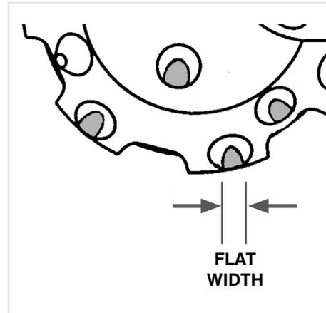
New tungsten carbide inserts work in compression where they are strong. As the carbide wears, flat spots appear leading to a horizontal or 'shear' load on the button.
