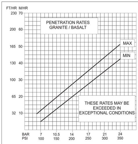
For example, if a hole diameter of 165 mm (6 1/2") and a penetration rate of 30 m/hr drilling in granite was needed, then an air pressure of around 17 bar (250 psi) would be necessary.
