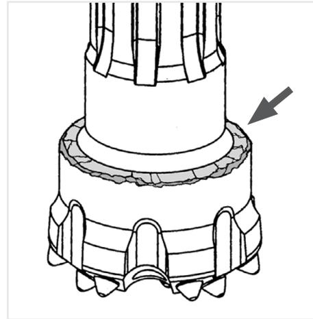
Shank breakage across the splines is generally caused by using a worn chuck, excessive torque or incorrect use of oversize drill bits.
