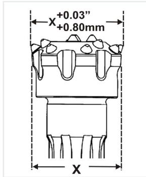
In highly abrasive conditions, the metal may wear more quickly than the carbide inserts. This is known as 'body wash' and in order to minimise carbide breakages, the carbide should be ground so that it does not protrude more than 9mm (0.35") above the metal surface.
