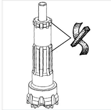
Shank breakage across the shank retaining ring diameter is generally caused by lack of lubrication or worn bit retaining rings, bit guide bush or bottom spacer.
