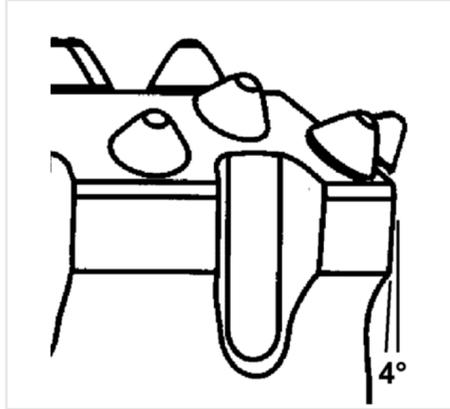
Ensure that the depth of flushing grooves is adequate and re-grind them regularly to allow free evacuation of the drilling debris.
