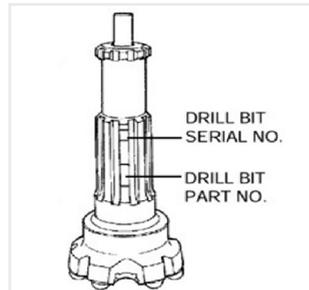
Inspect the drill bit, before use for any damage which may have occurred during transportation and prior to commissioning, take a note of the drill bit part number and serial number for future reference.
