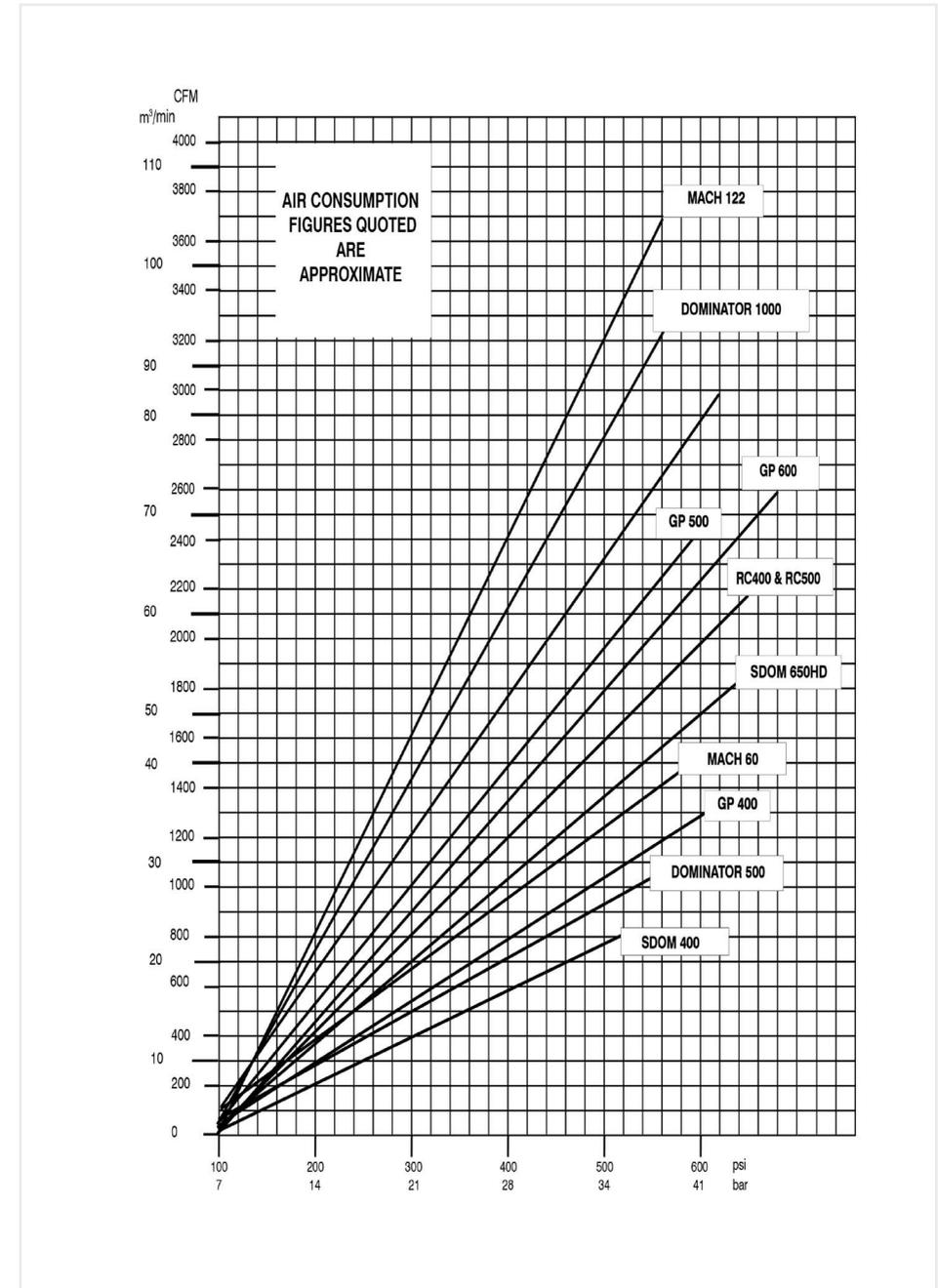
In selecting any air compressor capacity, the compressor therefore ideally should have a volume equivalent to the hammer air consumption at the required output pressure plus a minimum extra volume of 20% for contingency purposes.
