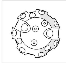
Excessive feed force can cause cracks on the face of the drill bit which can lead to large pieces of metal breaking off.
