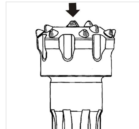
Broken inserts are generally caused by overdrilling the drill bit before reconditioning, reaming the hole, using excessive feed force or where there are existing tungsten carbide or other metal particles in the hole.
