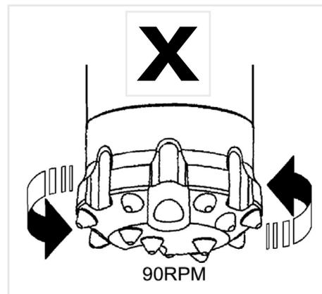
Face buttons which are flat generally indicate a lack of hammer blow energy or insufficient thrust.
