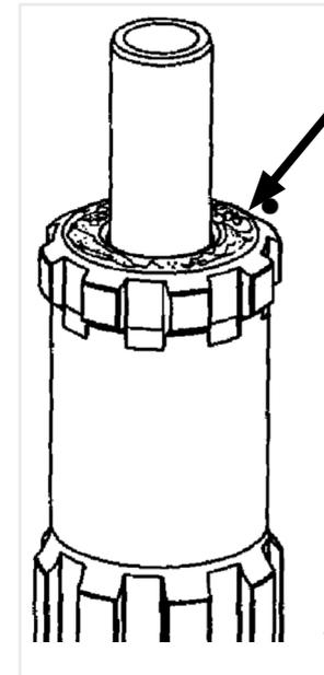
Ensure that the foot valve is not broken. This is generally caused by a worn piston or cylinder bore causing misalignment, lack of lubrication causing pick up or corrosion of water.
