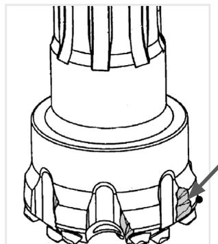
Re-drilling caused by poor hole cleaning and also high abrasion can result in deformation around the edges of exhaust holes and flushing grooves. These should be ground to ensure a clean obstruction free passage for exhausting air.
