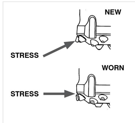
Rotating the bit faster than necessary will not generally increase penetration speed but it will increase the wear rate, particularly in abrasive rock.
