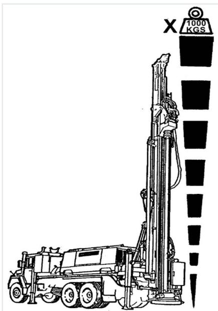
The above factors combine to reduce the amount of lifting power available for drill tubes and consequently the achievable drilling depth with any particular drill rig.
