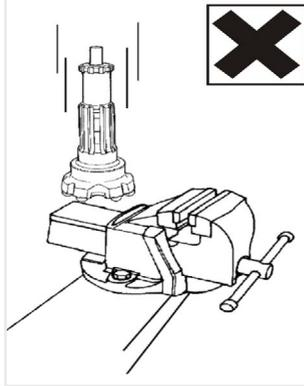
Ensure that drill bits (particularly tungsten carbide buttons) do not come into contact with a metal surface.
