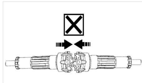
Do not allow tungsten carbide buttons to come into contact with each other.
