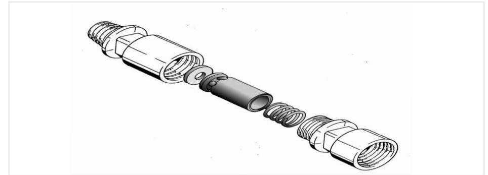
Most makes of hammers are offered with internal non-return valves for drilling under water but in addition to these, INTERTUBE NON-RETURN VALVES are available as an extra precaution to prevent internal contamination of the hammer and are fitted to the top of the drill string once water is encountered in the hole and not before.
