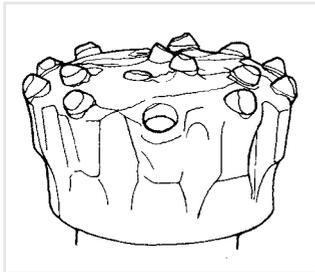
If the head is unevenly worn, the most likely causes are incorrect regrinding, bent drill tubes or drill string not being centralised in the drill rig table.
