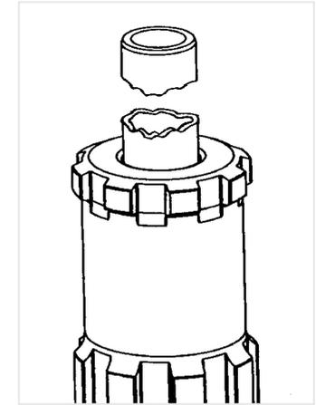
A broken striking end is caused generally by a badly worn piston, chuck, bottom bush or retaining ring.
