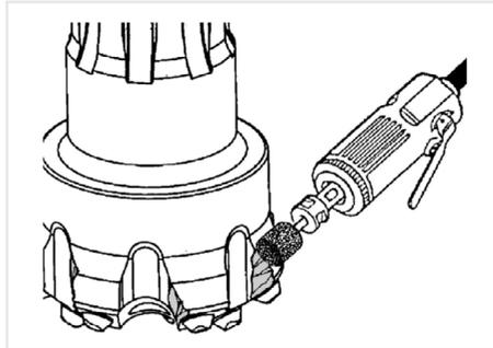
Ensure that the flushing holes are not deformed and grind them if necessary.
