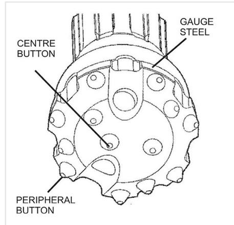
In abrasive conditions, it is advisable to monitor the rate of wear over a measured depth drilled to determine the frequency of re-grinding necessary. It is recommended that flat widths should generally not exceed 25% of the button diameter although this varies from manufacturer to manufacturer.
