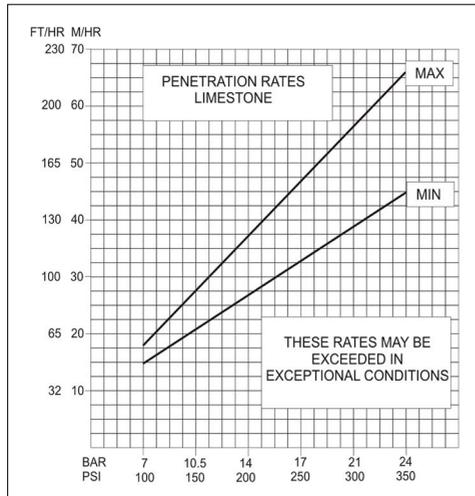
Penetration rates are generally dictated by air pressure. The higher the air pressure the faster the hammer will drill.
