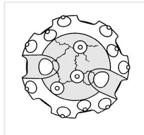
The depth of flushing grooves must be monitored as abrasion and/or high RPM wears away the drill bit body. The grooves must be regularly ground to ensure that drilling debris can adequately escape.
