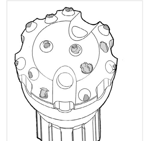
A DTH button bit can continue to drill with one or more broken buttons, but at a reduced penetration rate. Broken buttons should be ground off to prevent additional button particles breaking off and damaging other buttons.
