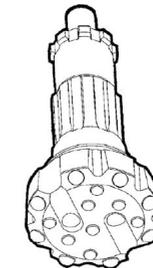
In the late 1960's however, the button bit was introduced and this was a landmark in the progress of DTH equipment which led to bit lives previously unheard of.
