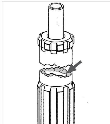
Damage to the shoulder is usually caused by excessive or insufficient thrust.
