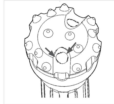
High levels of body wash and energy produced by the piston striking the drill bit can cause buttons to be hammered out of the bit body. This is known as button 'pop-out'. Button 'pop-out' can also occur even in drill bits with little body wash, where drilling in very soft conditions is being carried out and constant flushing is necessary because the drill bit face is not in constant contact with the bedrock.
