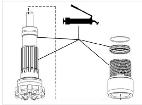
Before assembling into the hammer, ensure that the drill bit splines are thoroughly greased.
